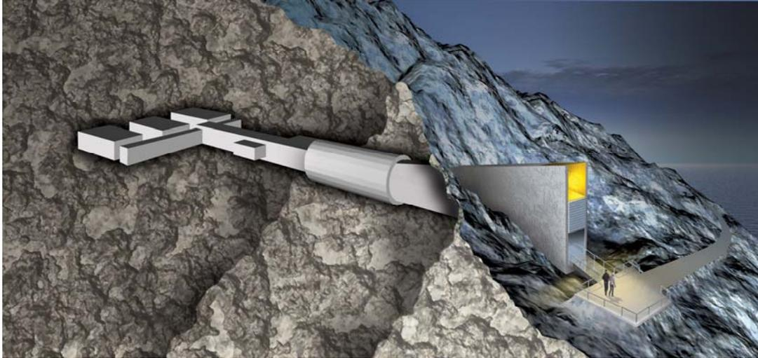
Fig. 1. The entrance of SGSV and a cross-section of the seed vault deep inside the mountain.
