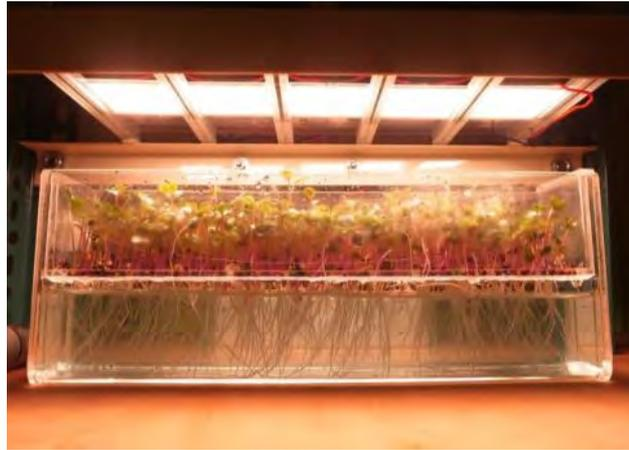
Fig. 1 Photo of experimental setup of sprout production using OLEDs
